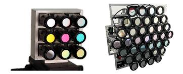
While the sensor and the lens stays the same for all cameras, the filter changes to record different parts of the light spectrum. For example, there are filters in the visible wavelength area to record an RGB image, but also in the infrared, which is often very helpful for classification of materials, since many materials have specific spectral absorption bands and therefore spectral fingerprints, which can be exploited to discriminate them.
